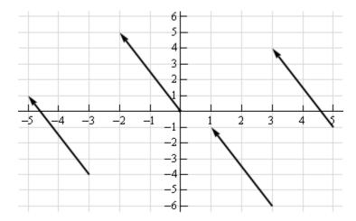
Each of the directed line segments in the sketch represents the same vector. In each case the vector starts at a specific point then moves 2 units to the left and 5 units up. The notation that we'll use for this vector is,
